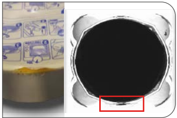
ACQUISITION EXAMPLE AND REAL DEFECTIVE PRODUCT
