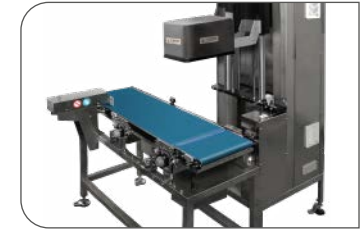
CONFIGURATION UPPER SIDE INSPECTION
